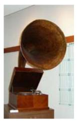
Made in England in 1935. This electric phonograph used 2 need b types, bam boo and steel. The bam boo need b was well suited for listening to recordings of reed instruments, and it could create a very warm, natural sound. The steel need b was better at reproducing the sounds of brass instruments such as the trumpet and trom bone. You can hear the sharper sounds created by the steel need b.
